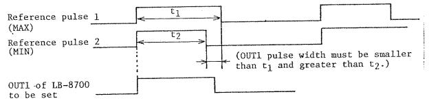
A reference circuit is used to indicate, by a lamp, for example, that the width of OUTl pulse has become smaller than  $t_1$  and greater than  $t_2$ . Use of measuring instrument is not needed, and the setting operation is possible at room temperature.
