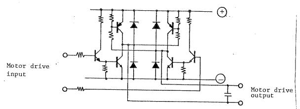
Basically the motor drive circuit should be such a transistorized one as that shown above.
